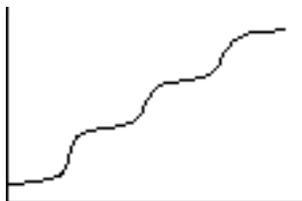
a.  $\text{H}_2\text{CO}_3$  titrated with NaOH
