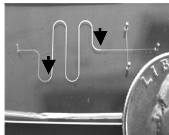
Figure 4. Sample PDMS chip packed with C18 beads compared to a U.S. quarter. Channel length within arrows shows packing of beads.
