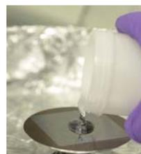
Figure 3. PDMS being poured onto the mold to form chip.
