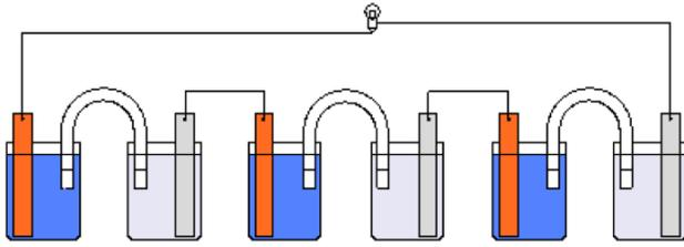
**Figure 8 - Battery of three Daniell's Cells**
