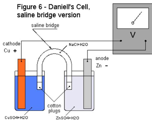
this battery can be represented using the line diagram as:
